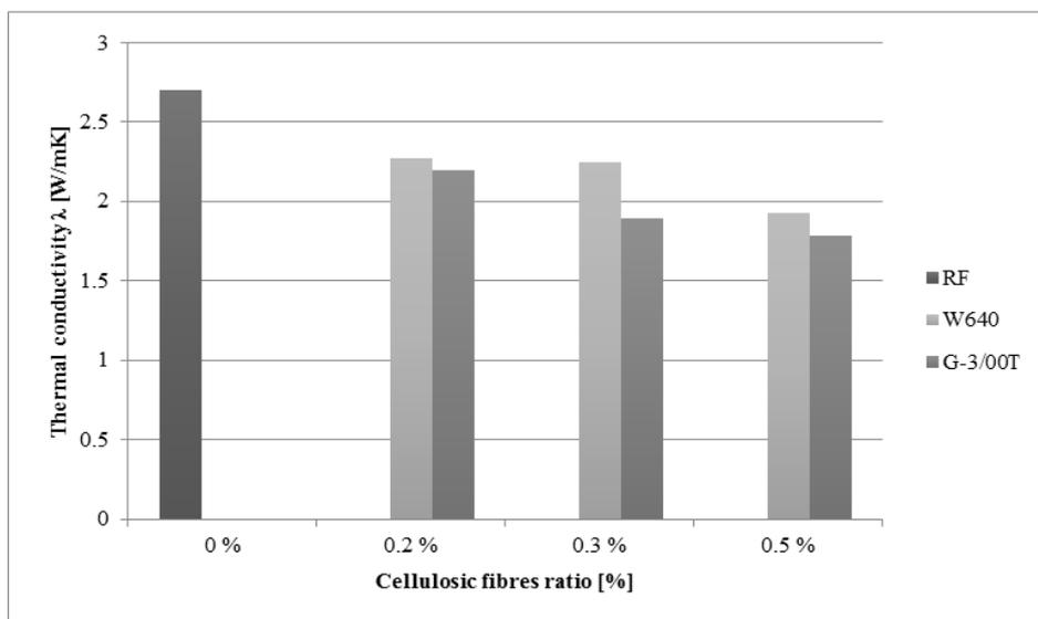
Fig. 6. Dependence of thermal conductivity on cellulosic fibre content
