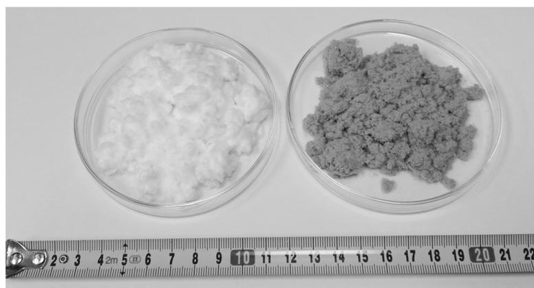
Fig. 1. Cellulosic fibres Grencel from wood pulp W640 (white) and waste paper G-3/00T (grey)
