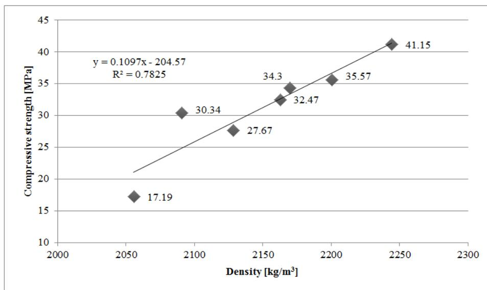
Fig. 4. Relationship between compressive strength and density of fibre cement composites after 28 days of curing
