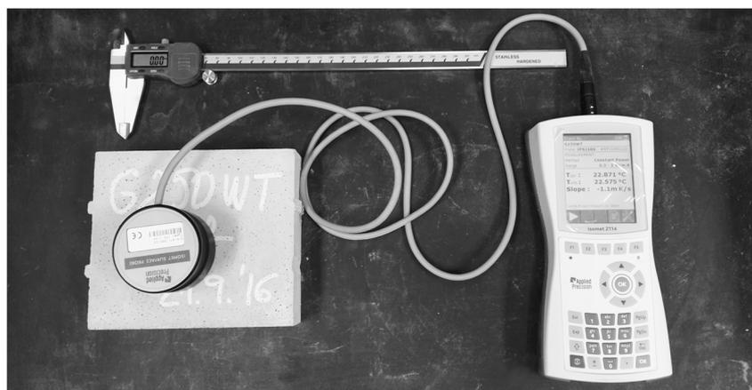
Fig. 2. Measurement of thermal conductivity coefficient of cement plaster reinforced with cellulosic fibres
