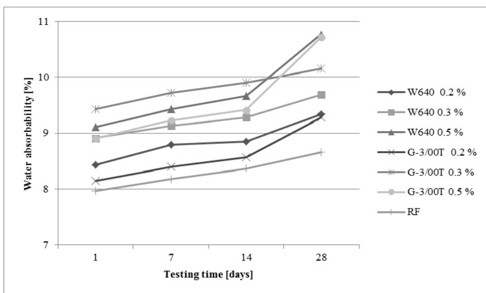
Fig. 5. Development of water absorbability of fibre cement composites in time
