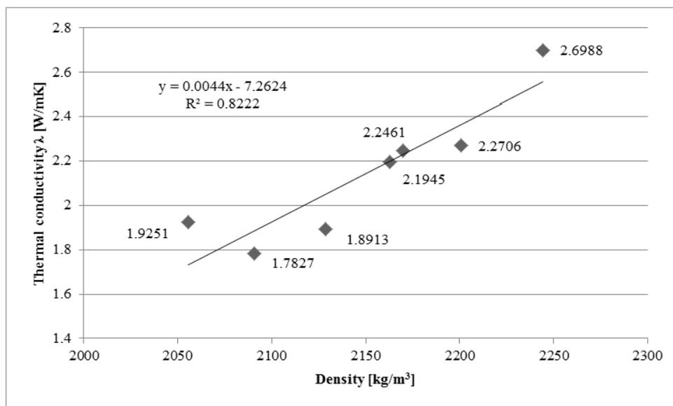
Fig. 7. The relationship between the thermal conductivity coefficient and density after 28 days of curing
