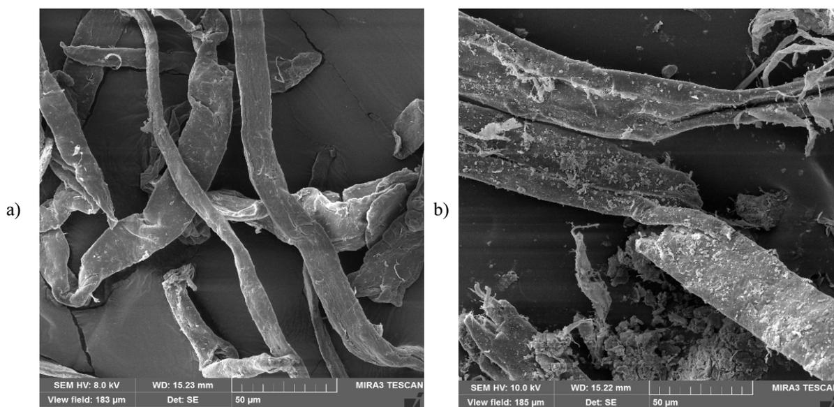
Fig. 3. SEM image of a) wood pulp fibres W640 at magnification 1500 times and b) recycled waste paper fibres G-3/00T at magnification 1500 times
