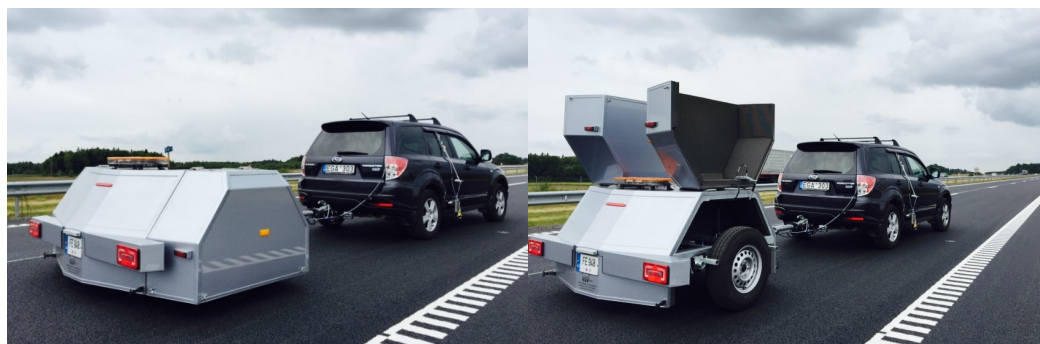
Fig. 3. CPX noise level measurement trailer (left – closed; right – opened)
