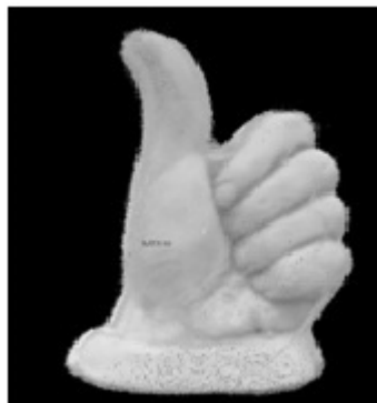
Fig. 6. The point clouds of the hand obtained in Leica Cyclone program
