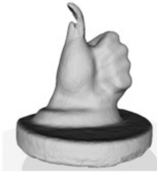
Fig. 8. Hand model obtained using the Sensor Kinect device
