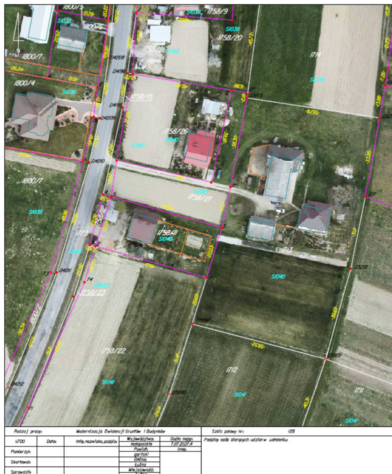
Fig. 5. Boundary contour from determining the boundaries in Lužna cadastral district
