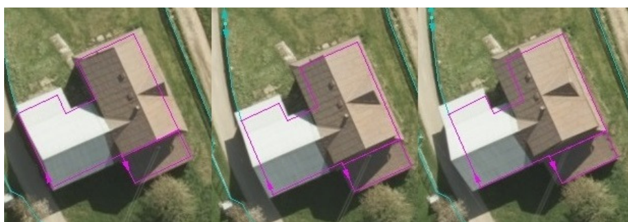
Fig. 3. Apparent displacement of the contour of the building relative to the model – example 2
