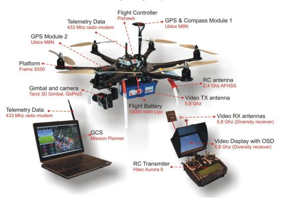
Fig. 2. Hexacopter platform hardware configuration and components assembly
