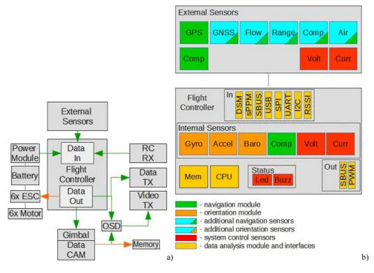
Fig. 1. The hexacopter platform's hardware modules internal communication (a) and (b) flight controller modules and communication ports
