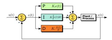
Fig. 3 PID controller to hexacopter (Liang 2017)
