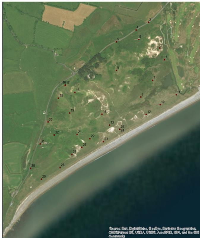
Fig. 3. Ground control points map for UAV surveying
