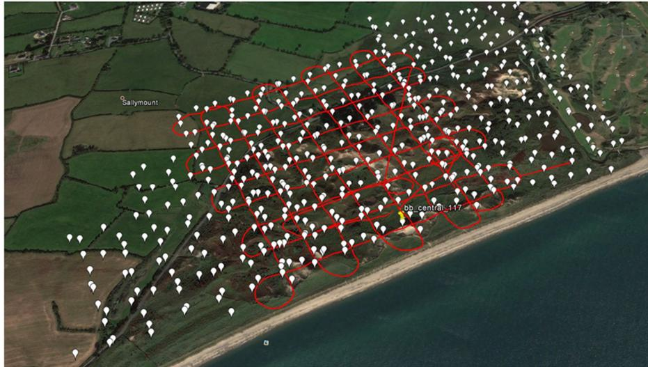
Fig. 4. Flight path for UAV surveying at three sections of study site
