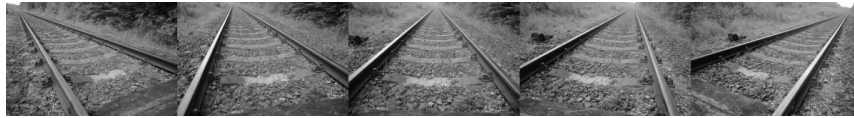
Fig. 1. Configuration of 5 terrestrial oblique – convergent photos in one example strip of the tested object (source: own elaboration)
