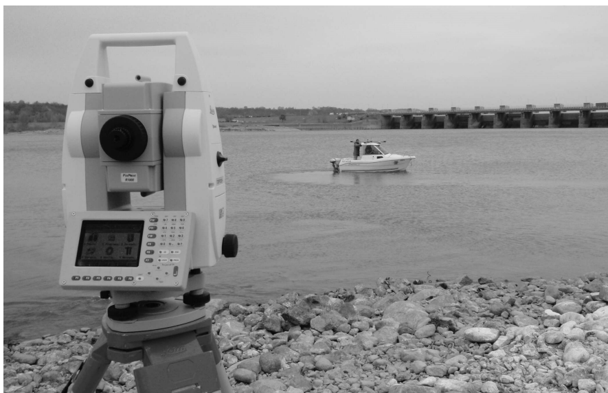
Fig. 4. The hydrographic boat during RTS positioning
