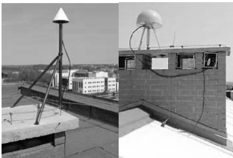
Fig. 1. The stabilization of the stations selected for the research ( www.asgeupos.pl ), left – ELBL, right – OLST
