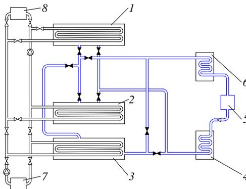
Fig. 4. Cascade adsorption refrigeration unit 1 – adsorber filled with zeolite 2 – adsorber filled with zeolite, 3 – adsorber filled with silica gel, 4 – evaporator, 5 – refrigerant tank, 6 – condenser, 7 – heat source, 8 – heat sink
