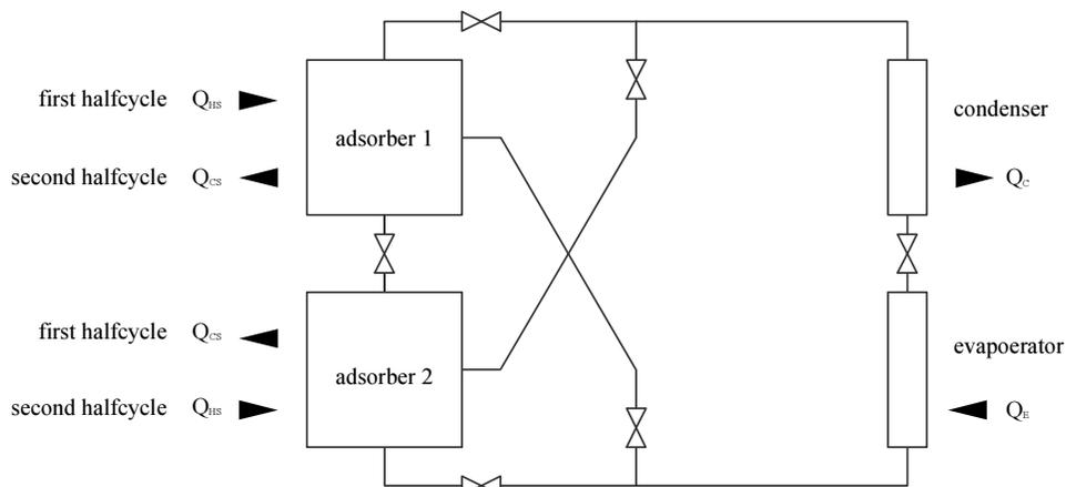
Fig. 1. Two beds adsorption refrigeration unit
