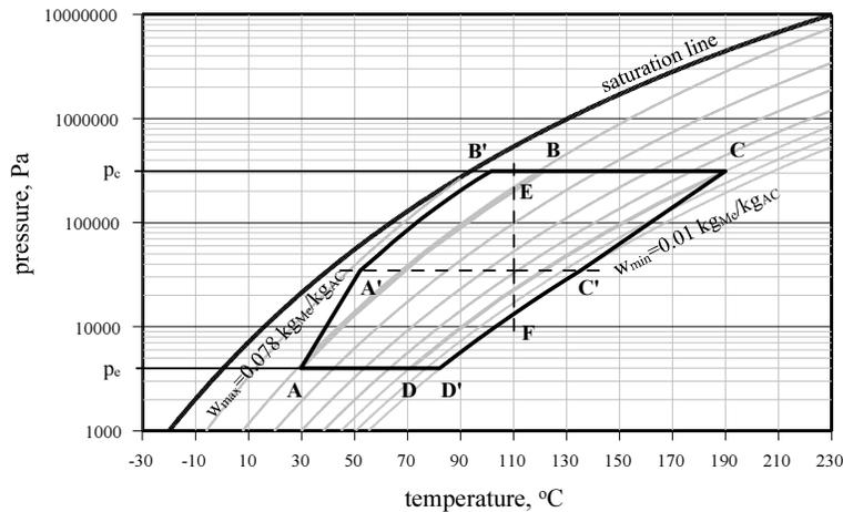
Fig. 3. Heat and mass recovery in two beds adsorption unit
