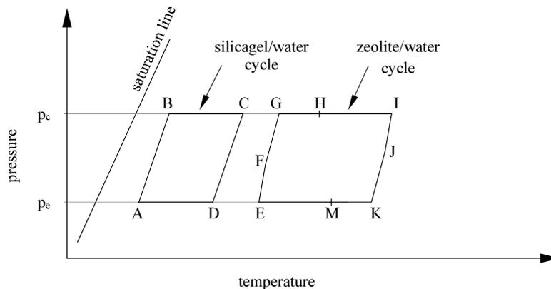
Fig. 5. Thermodynamic states of beds for cascade adsorption refrigeration system
