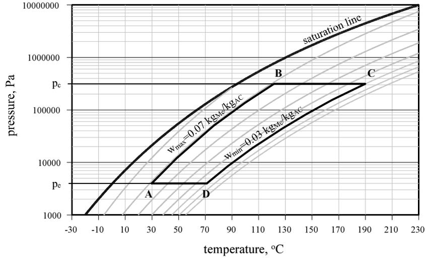
Fig. 2. Adsorber beds states during operation
