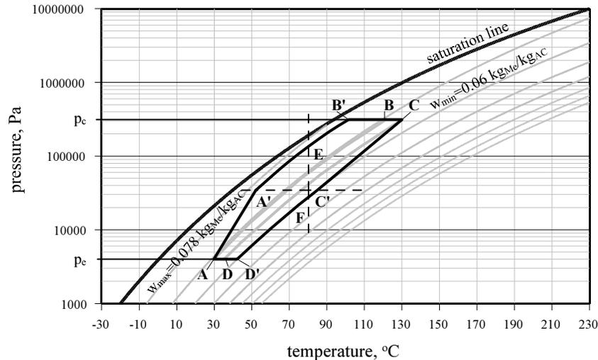
Fig. 6. The potential of heat and mass recovery for lower driven temperatures
