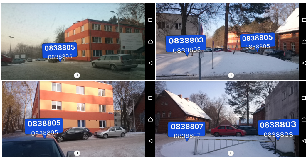
Fig. 6. Approximate location of geodetic control points presented in AR mobile application (source: own work)
