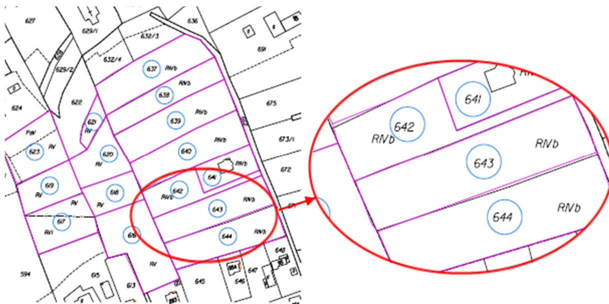
Fig. 2. The resulting map (scale 1: 2000) of the measured complex of plots showing the differences in the course of borders
