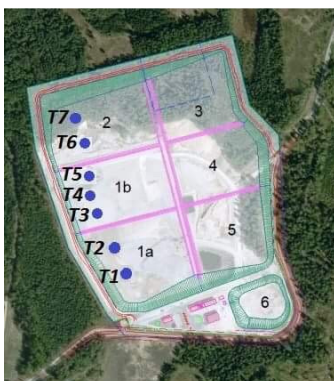
Fig. 1. Section of the Kazokiškės landfill: 1a, 1b – filled sections; 2 – almost filled section; 3–6 – future sections (yet to be set up); T1–T2 – air sampling sites
