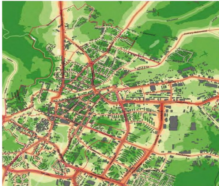
Fig. 2. The map of noise developed in the framework of the Municipal Programme of Revitalisation of Olsztyn Source: www.msipmo.pl
