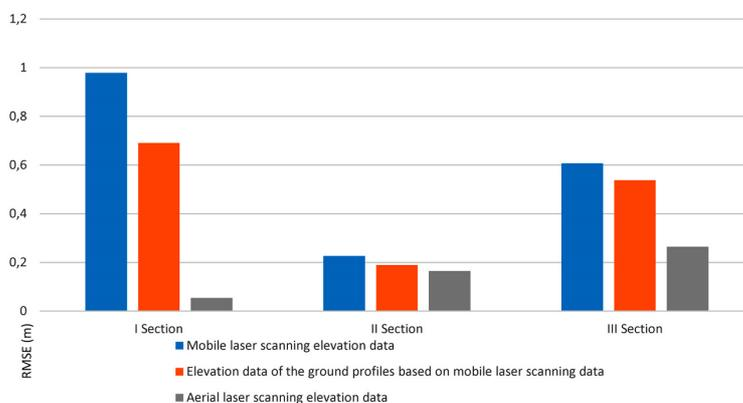
Fig. 6. Comparison of elevation data RMSE's using different measuring methods in sections I, II and III
