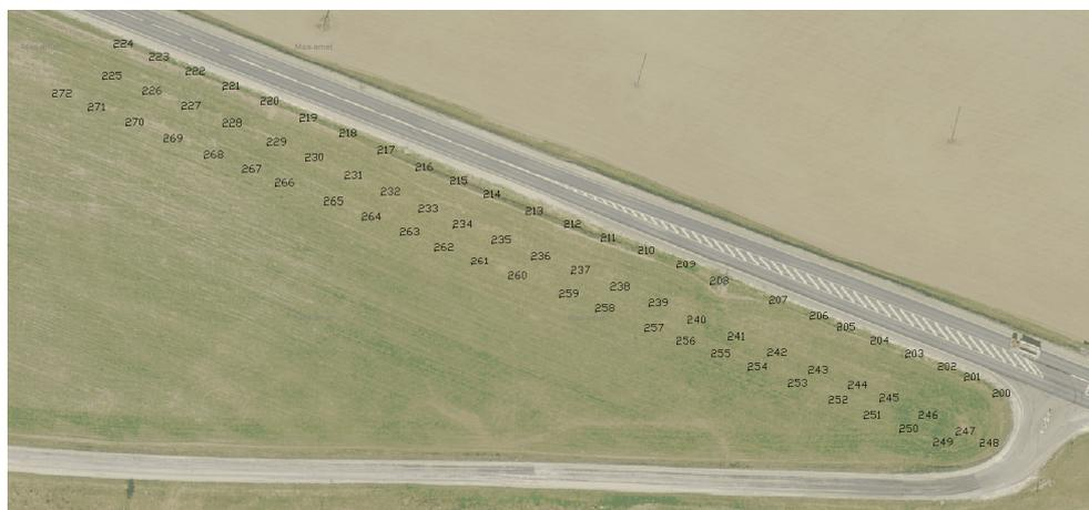
Fig. 4. The layout of checkpoints measured with a GNSS device on section I
