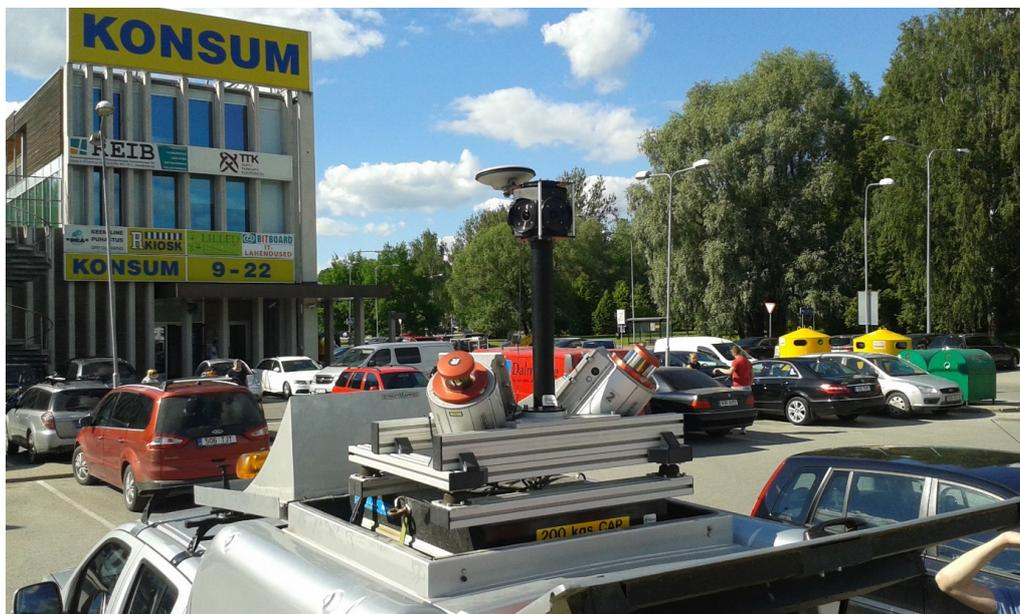
Fig. 2. Mobile laser scanning system StreetMapper 360
