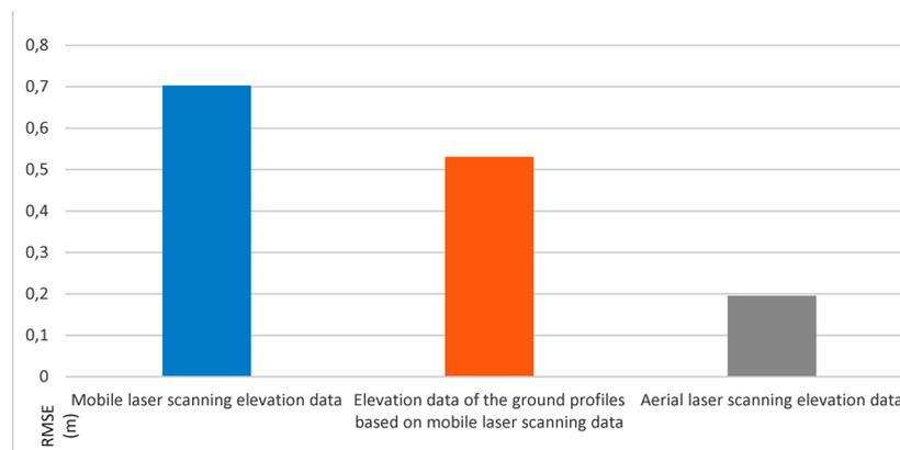
Fig. 7. Comparison of mean elevation data RMSE's of all the sections using different measuring methods
