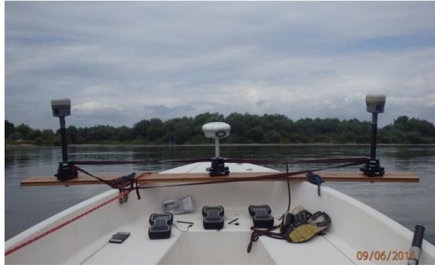
Fig. 2. The bathymetric boat during the measurement on the Vistula river
