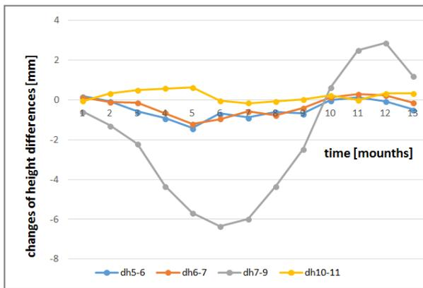
Fig. 7. Trajectories of changes in height differences based on measurements (Source: own elaboration)
