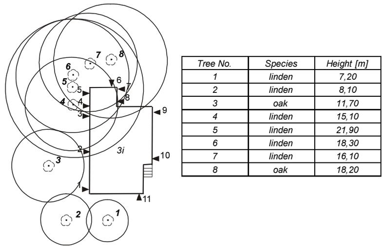
Fig. 6. Location of the measurement points on the building and the location of the trees (Source: own elaboration)
