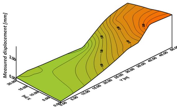
Fig. 13. Prediction of vertical displacements for the measurement period of July 2015 (Source: own elaboration)
