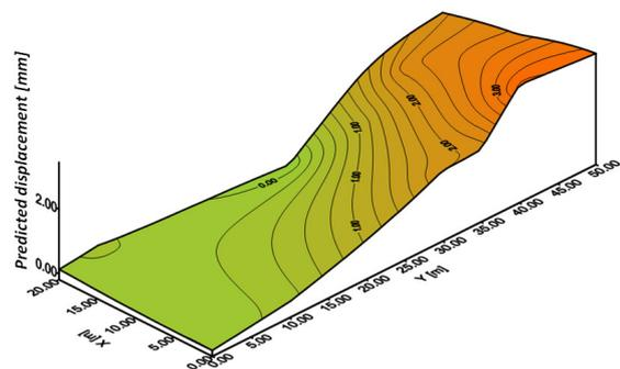
Fig. 14. Displacements actually measured in July 2015 (Source: own elaboration)
