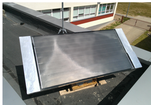
Fig. 1. SAH tested experimentally in normal operating conditions
