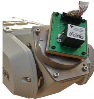
Fig. 4. Robot head with ADIS
