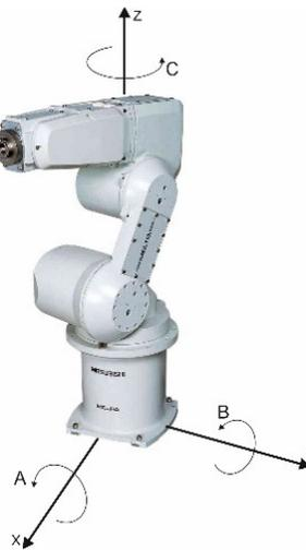
Fig. 2. Coordinate system of a robot (MITSUBISHI 2009)
