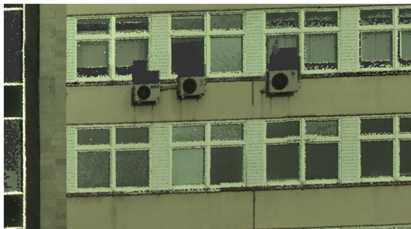
Fig. 4. The lack of data in shadowed places
