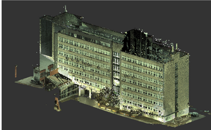
Fig. 3. RGB colored point cloud representing building of Vilnius Gediminas Technical University Faculty of Environmental Engineering
