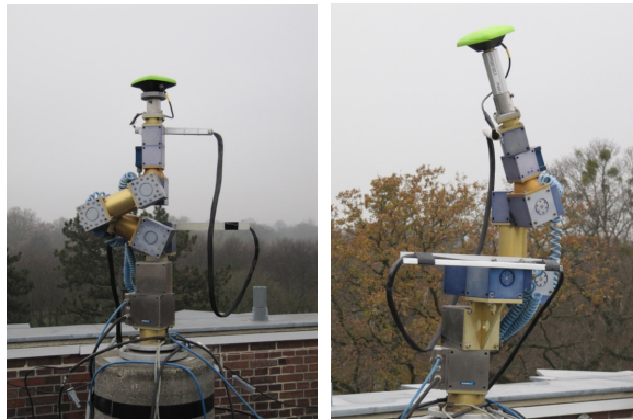
Fig. 1. JAV_GRANT-G3T calibration: without a spacer (left) and with a 120 mm spacer (right)
