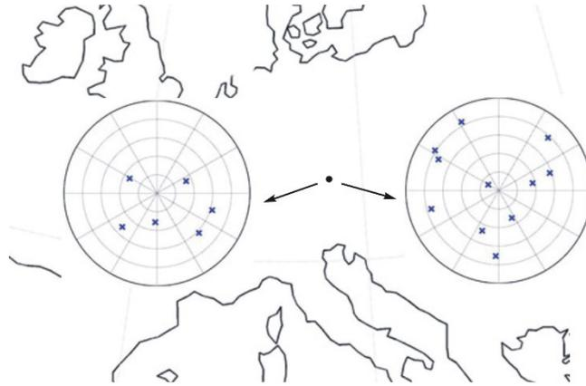
Fig. 4. Skyplot of GPS constellations as used in the simulations, two scenarios; average: PDOP = 2.5 (left) and good: PDOP = 1.7 (right)
