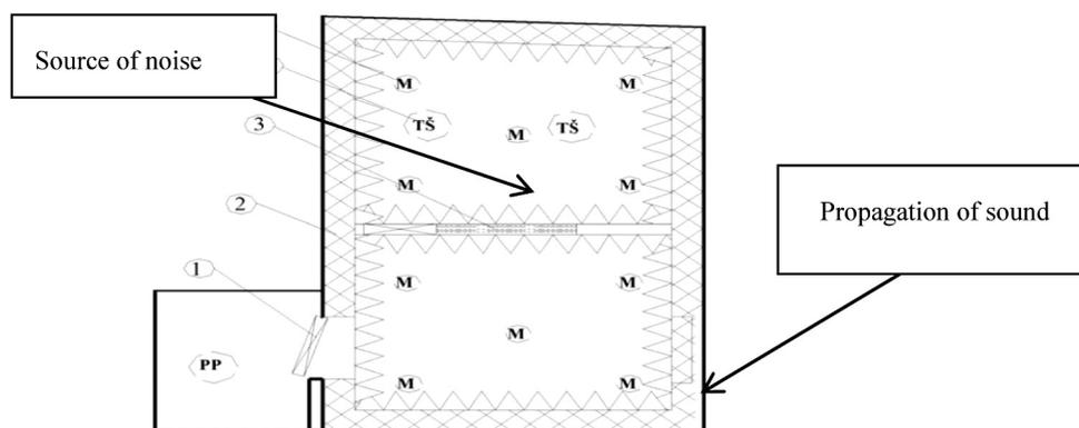
Fig. 3. Situation plan of the noise-suppression chamber: a) view from above the noise-suppression chamber: 1 – door; 2 – chamber partitions covered with foam; 3 – cage for mounting the study samples; 4 – positions of noise sources (TŠ); 5 – microphone positions (M); PP – data-recording-and-processing room (Grubliauskas, Butkus 2009)
