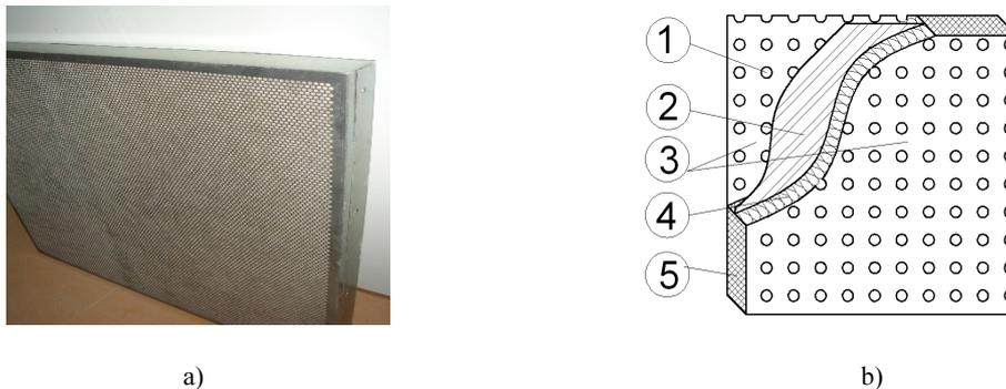
Fig. 6. A perforated tin shield with a filler: a) view of the construction; b) layer of the construction
