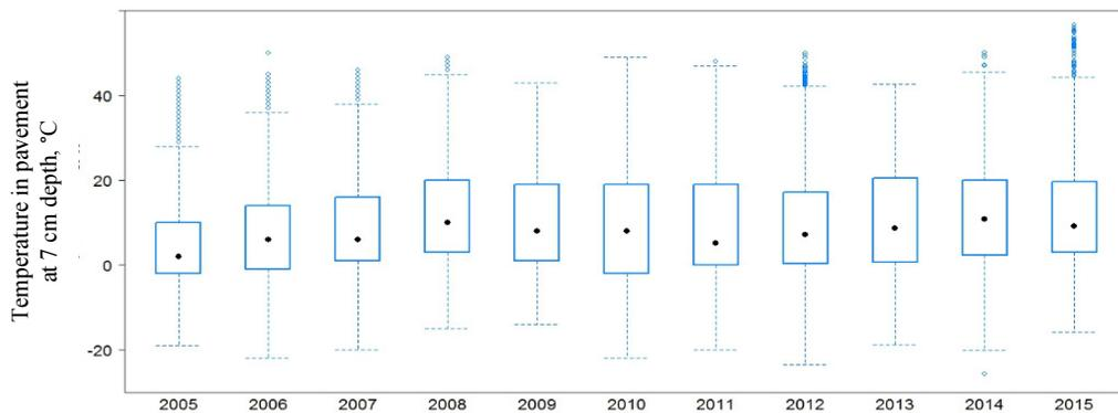
Fig. 4. Pavement temperature variation per year measured at 7cm depth
