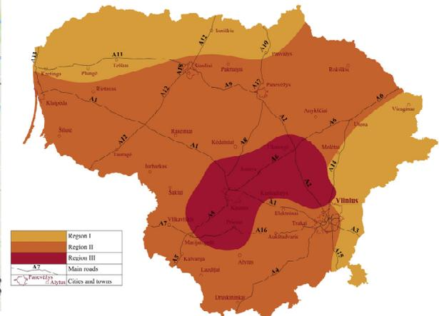
Fig. 8. Classification of Lithuania based on surface and pavement temperature analysis
