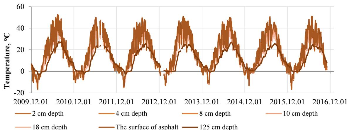
Fig. 1. Recorded temperature variation during 2009–2016 (Source: Žiliūtė *et al.* 2016)
