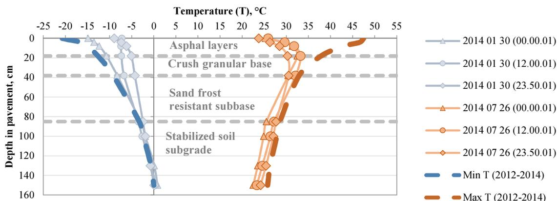
Fig. 2. Measured temperature profiles in REPS (No. 18)
