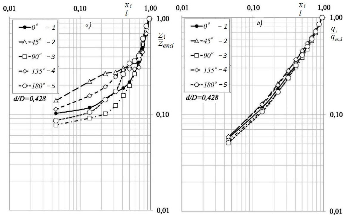
Fig 5. Distribution of operating heads along CP (a) and distribution of water inflow into CP through individual input nozzles along the path (b) for CP whose angles  $\beta$  and Reynolds criteria are corresponded equal to the following:
