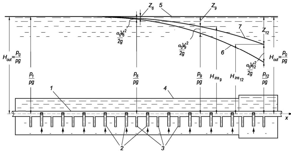
Fig. 4. Schematic diagram for calculation of full operating head in CP: 1 – CP investigated; 2 – input nozzles; 3 – connection pipes for connection of pulls lines from piezometers; 4 – transparent cylinder for CP; 5 – water level which corresponds to the head in the transparent cylinder; 6 – piezometric line for water stream inside CP; 7 – ditto, line of full operating head; x – axis of CP (Cherniuk, Ivaniv 2017)
