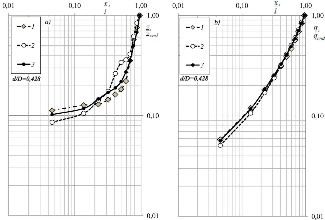
Fig 6. Distribution of operating heads (a) in different CPs and that of water inflow in them (b): 1 – combined CP for which the first five nozzles are with  $\beta = 0^\circ$ , and the other six nozzles with  $\beta = 180^\circ$  for  $Re_D = 7242$ ; 2 – CP with  $\beta = 180^\circ$ ,
