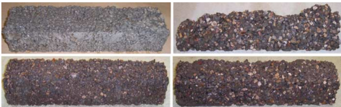
Fig. 5. Some examples of pervious concrete freeze thaw testing (source: Kevern et al. 2008)
