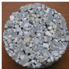
Fig. 1. Cross section of pervious concrete cylinder
