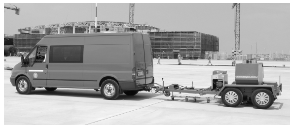
Fig. 2. HWD when measuring the airport pavement deflections
