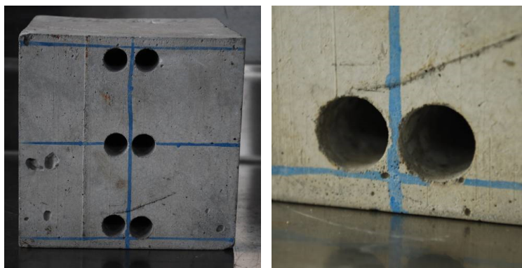
Fig. 2. The way of collecting cores from concrete samples
